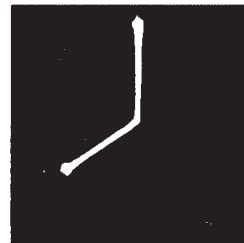
Diode parallel 680Ω
